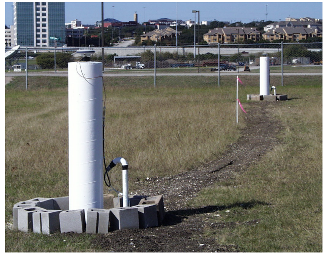
Figure 4 Survey monuments at ARL:UT used to characterize BSS antenna PCO.
